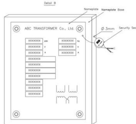
Note : The hole shall be drilled by manufacturer and thread with security seal by PEA
