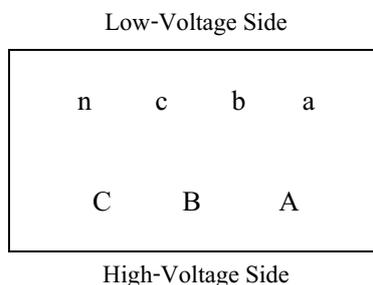
**Figure 6 315 -2,000 kVA Tank top view**
