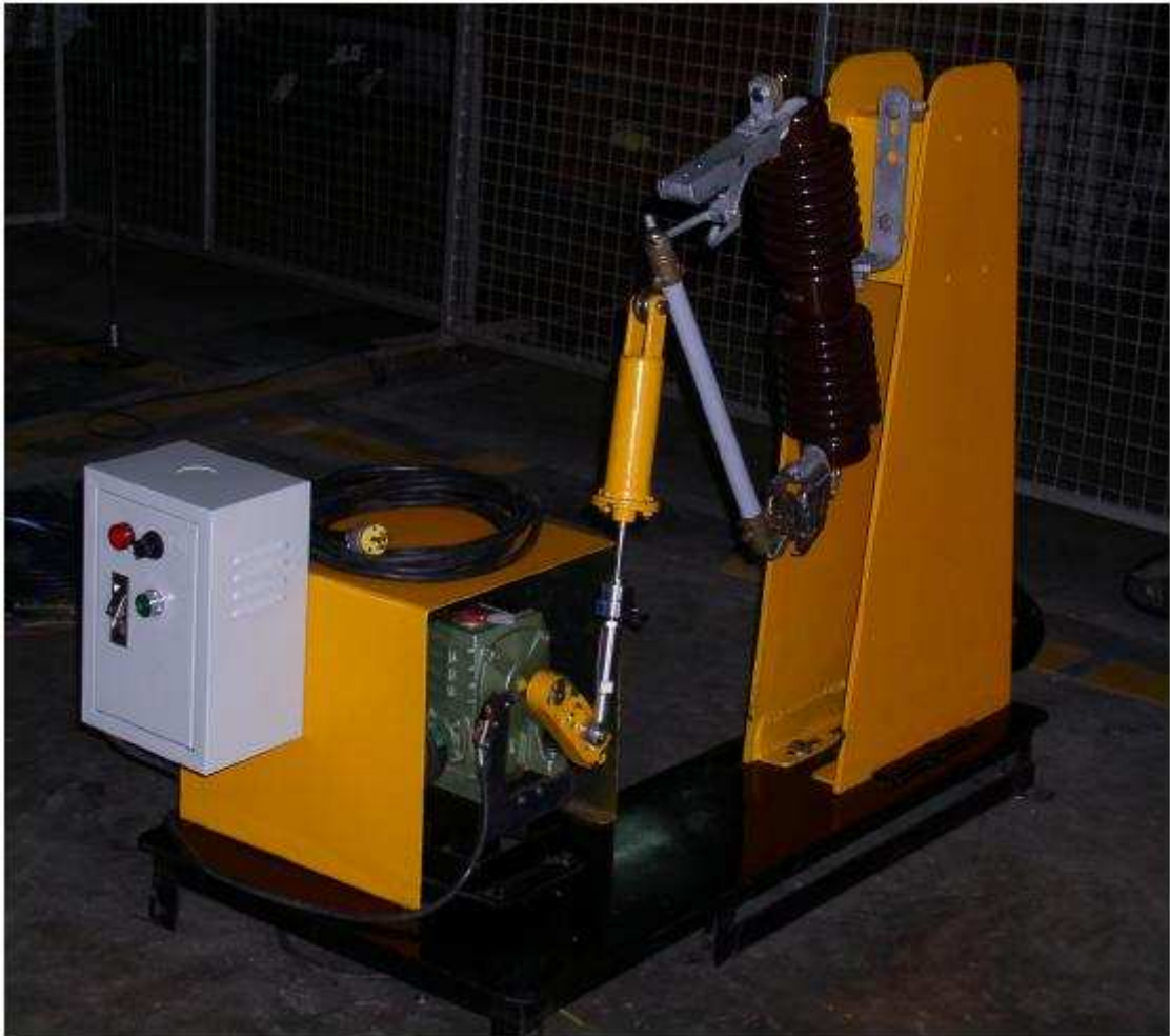
Fuse cutout closing machine
