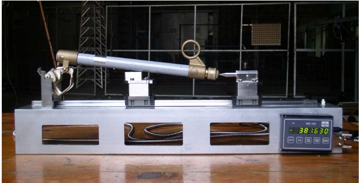
Fuse holder length measuring device
